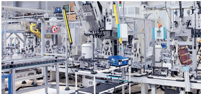
Systematic Safety Safety locks and safety light curtains can be connected via Safety Relays in order to provide comprehensive personal safety in assembly areas. The relays evaluate the signals generated by the interconnected components.
