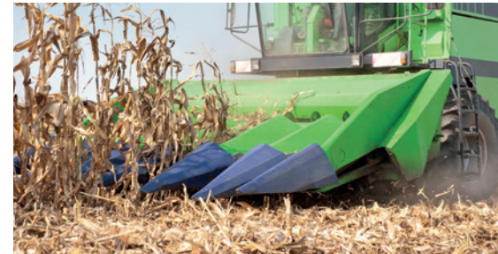
Agriculture Industry Ultrasonic sensors measure distance to the ground in dusty environments in harvesting machines, in order to prevent them from bottoming out and the resultant damage.
