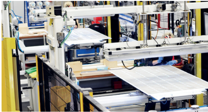
Securing Areas Safety light arrays provide optimized body protection by securing access to danger zones.
