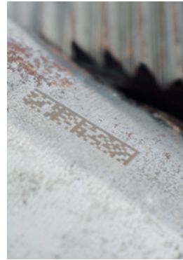
Automotive Industry 1D/2D code scanners read laser printed data matrix codes by means of which components can be identified and retraced after the manufacturing process (track & trace).
