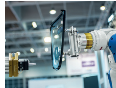
Automotive Industry In automobile production, ultrasonic sensors reliably detect transparent objects like windshields.
